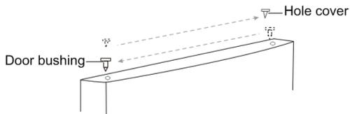
18. Remove the hole cover from the top left side of the cabinet and secure the cover on the top right side of the cabinet.
