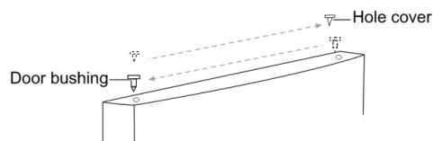
13. Remove the center hinge screw hole plug on the left side of the cabinet, then install in the screw holes on the right side of the cabinet.
