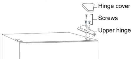
3. Remove the refrigerator compartment door from the cabinet.
