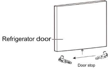
16. Install the Refrigerator compartment door.
