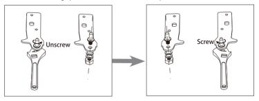
9. Install the hinge at left side and foot base at right side. Then screw two leveling feet with their original parts.
